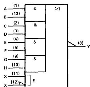
positive logic:  $Y = \overline{AB} + \overline{CD} + \overline{EF} + \overline{GH} + X$
