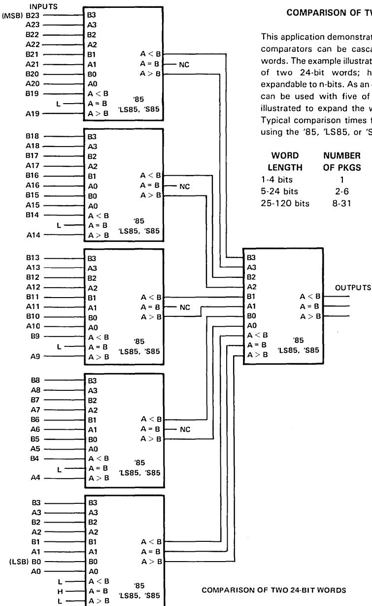
This application demonstrates how these magnitude comparators can be cascaded to compare longer words. The example illustrated shows the comparison of two 24-bit words; however, the design is expandable to n-bits. As an example, one comparator can be used with five of the 24-bit comparators illustrated to expand the word length to 120-bits. Typical comparison times for various word lengths using the '85, 'LS85, or 'S85 are:
