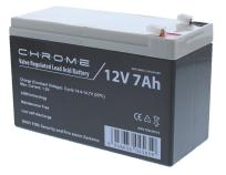
The rechargeable batteries are lead-lead dioxide systems. The dilute sulfuric acid electrolyte is absorbed by separators and thus immobilized .Should the battery be accidentally overcharged producing bydrogen and oxygen,Special one-way valves allow the gases to escape thus avoiding excessive pressure build-up.Otherwise,the battery is completely sealed and is,therefore, maintenance -free,leak proof and usable in any position.
