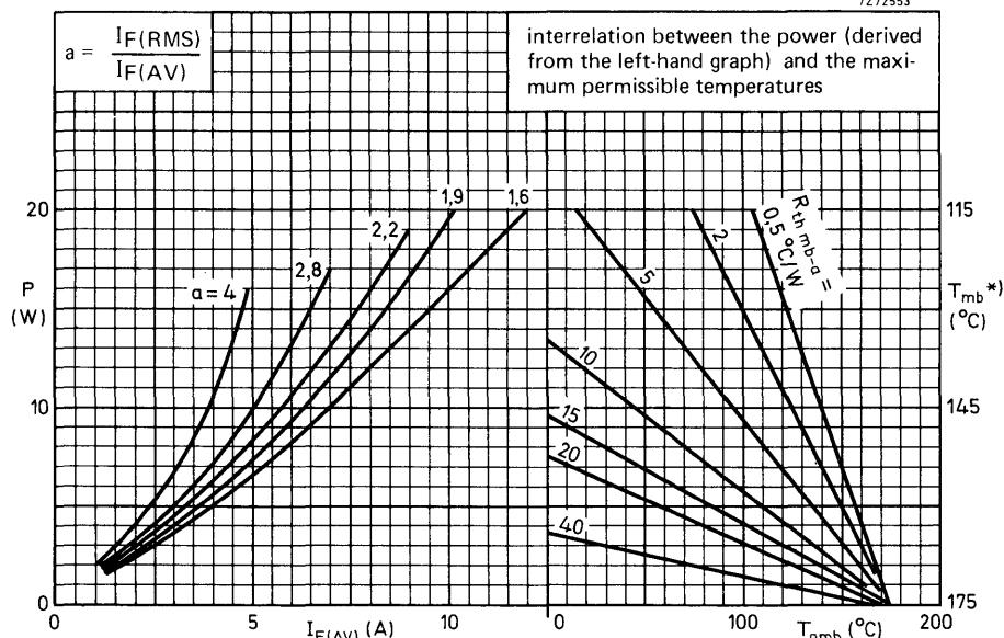
\*)  $T_{mb}$ -scale is for comparison purposes only and is correct only for  $R_{th\ mb-a} \leq 22\ ^{\circ}\text{C/W}$
